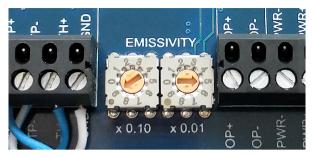
To adjust the emissivity setting:
