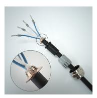
Ensure the cable shield braid is folded back over the cable jacket and gripped by the metal shield ring. This ensures a good electrical connection to the cable gland.  Thread the wires through the gland and re-connect them to the screw terminals.
