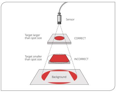
The size of the area (spot size) to be measured determines the distance between the sensor and the target. The spot size must not be larger than the target. The sensor should be mounted so that the measured spot size is smaller than the target.
