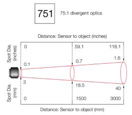
Diagrams show the diameter of the measured spot at each distance, for 90% energy.
