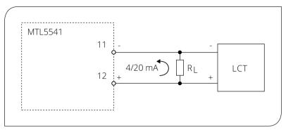
Configuration B: 180  $\Omega \le RL \le 580 \Omega$  (using the internal resistance)
