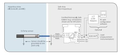
An alternative certified Intrinsically Safe isolator or safety barrier may be used. The connections shown above are for the suggested isolator, model MTL 5541.
