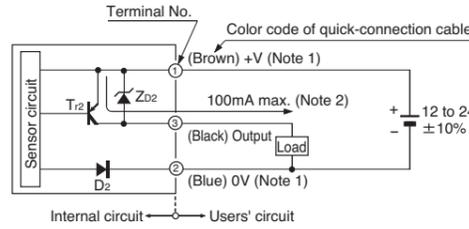
Notes: 1) The quick-connection sub cable does not have +V (brown) and 0V (blue). The power is supplied from the connector of the main cable.
