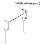
(Note1): When using the narrow beam type **EX-1**□**S**□, if the beam axes are out of alignment, check to see if the emitter and the receiver are facing each other in a straight line.
