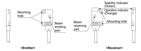
Thru-beam side sensing type: EX-11E□, EX-13E□, EX-19E□ EX-11SE□, EX-13SE□,
