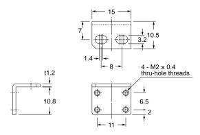
(Note):The sensor bracket is an object for satandard-beam type. It cannot be used for narrow-beam type.
