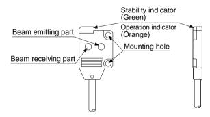
Thru-beam front sensing type with operation mode switch on bifurcation: EX-15, EX-17
