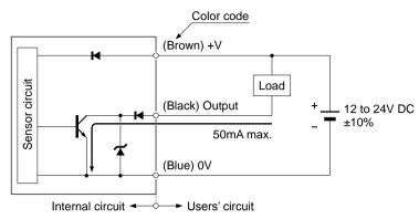
Note: The thru-beam type sensor emitter does not incorporate the output..
