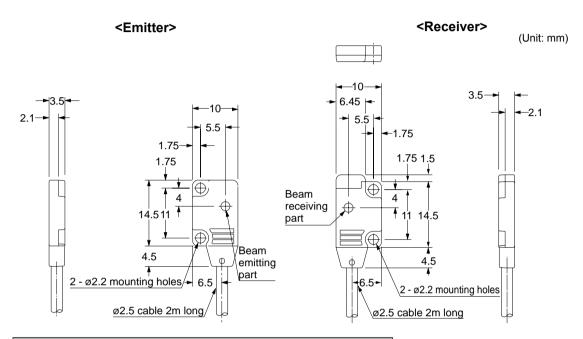
Thru-beam side sensing type: EX-11E□, EX-13E□, EX-19E□ EX-11SE, EX-13SE
