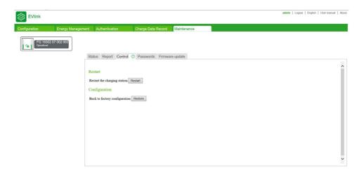
The **Restart** button restarts the charging station after a change to a parameter for example.
