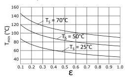
Graph showing the minimum measurable object temperature (Tmin), determined by surface emissivity (ε) and sensor temperature (TS).
