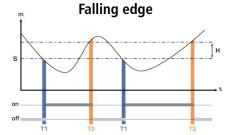
Measurement (m) < Threshold (S) during the timedelayT1: Alarm activation.
