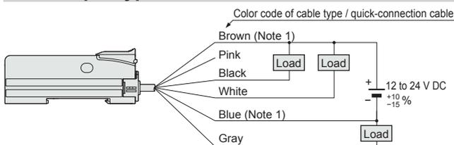
Notes: 1) The quick-connection sub cable does not have brown lead wire and blue lead wire. The power is supplied from the connector of the main cable.
