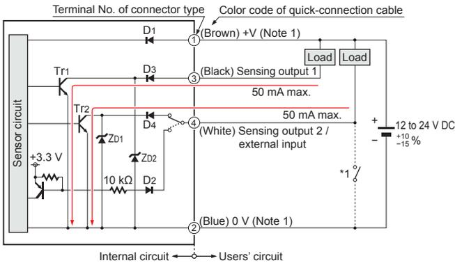
Notes: 1) The quick-connection sub cable does not have +V (brown) and 0 V (blue). The power is supplied from the connector of the main cable.
