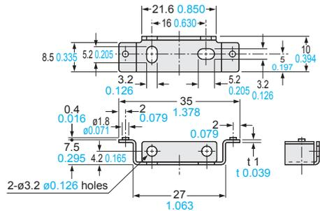
Material: Cold rolled carbon steel (SPCC)
