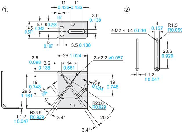
**MS-EXL2-1** Sensor head mounting bracket for LS-H102□ (Optional)
