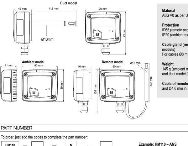
Ambient humidity transmitter HM110, active 0-10 V
