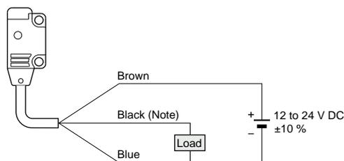
Note: The emitter of the thru-beam type sensor does not incorporate the black wire.
