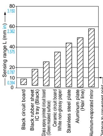
The bars in the graph indicate the sensing range (typical) for the respective material. However, there is a slight variation in the sensing range depending on the product. Further, if there is a reflective object (conveyor, etc.) in the background of the sensing object, since it affects the sensing, separate it by more than twice the sensing range shown in the left graph.
