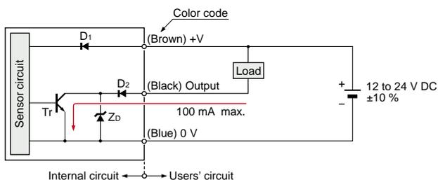
Symbols ... D1: Reverse supply polarity protection diode
