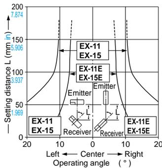
\*Optical properties of side sensing types (EX-□E□)
