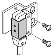
Tighten along with the sensor mounting bracket.
