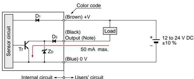
Note: The emitter of the thru-beam type sensor does not incorporate the output.
