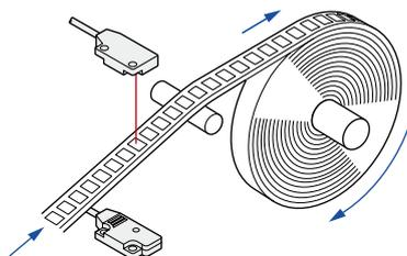
**Minimum sensing object:  $\varnothing 1\text{ mm}$   $\varnothing 0.039\text{ in}$  EX-11(E), EX-15(E)**
