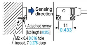
The tightening torque should be 0.2 N·m or less.
