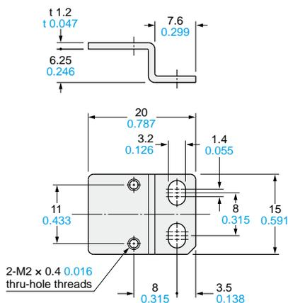
Material: Cold rolled carbon steel (SPCC)
