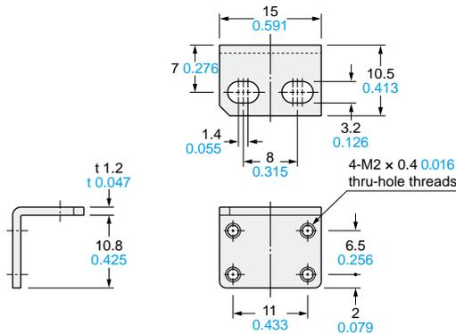
Material: Cold rolled carbon steel (SPCC)
