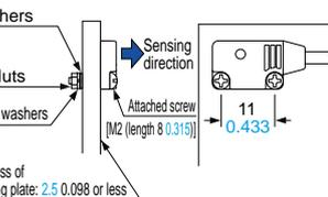
The tightening torque should be 0.2 N·m or less.
