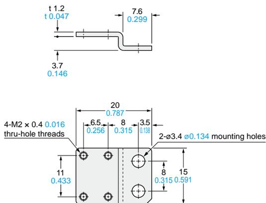
Material: Cold rolled carbon steel (SPCC)
