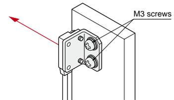
Note: Sensor mounting brackets can not be used for the narrow beam type (EX-□S□).
