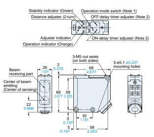
Notes: 1) The operation mode switch of the DC-voltage type is the DIP switch.
