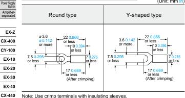
Note: Use crimp terminals with insulating sleeves. Recommended crimp terminal: Nominal size 1.25 × 3.5 0.049 × 0.138.
