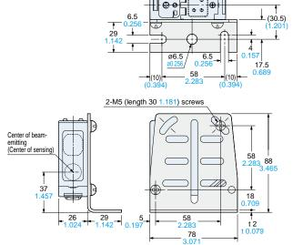
Material: Cold rolled carbon steel (SPCC)
