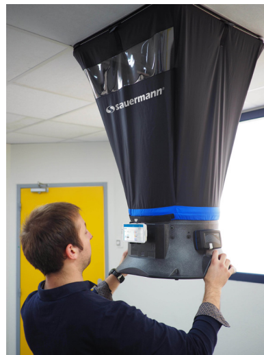
Use of the air flow meter
