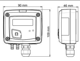
Material: ABS V0 as per UL94 Protection: IP65 Display: LCD 10 digits. Size: 50 x 17 mm Height of digits: Value: 10 mm; Unit : 5 mm Connections: ribbed, Ø6.2 mm Cable gland: for cables Ø8 mm maximum Weight: 143 g
