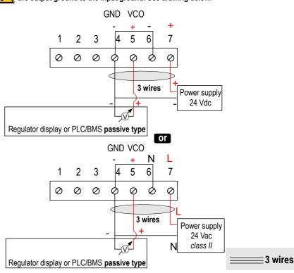
For CO110-P models with 4-20 mA output - passive:
