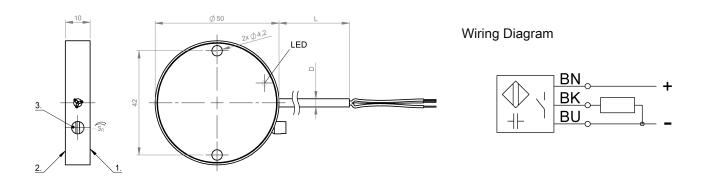
1) Sensing surface 2) Housing 3) Potentiometer 4) LED function indicator
